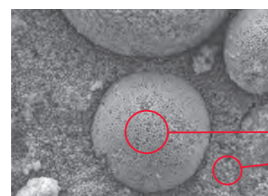
SEM Image of OMNICHROMA at 5,000x Magnification
